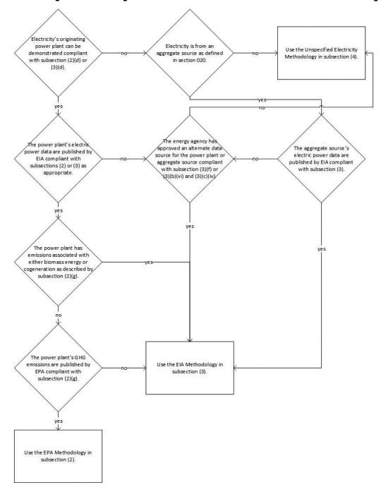
Figure 1: Simplified representation of the method selection process
